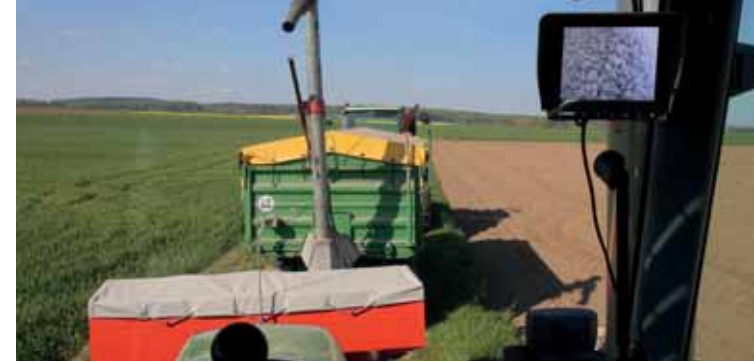
Top: Camera-monitored fill level indicator Bottom: Track monitoring
