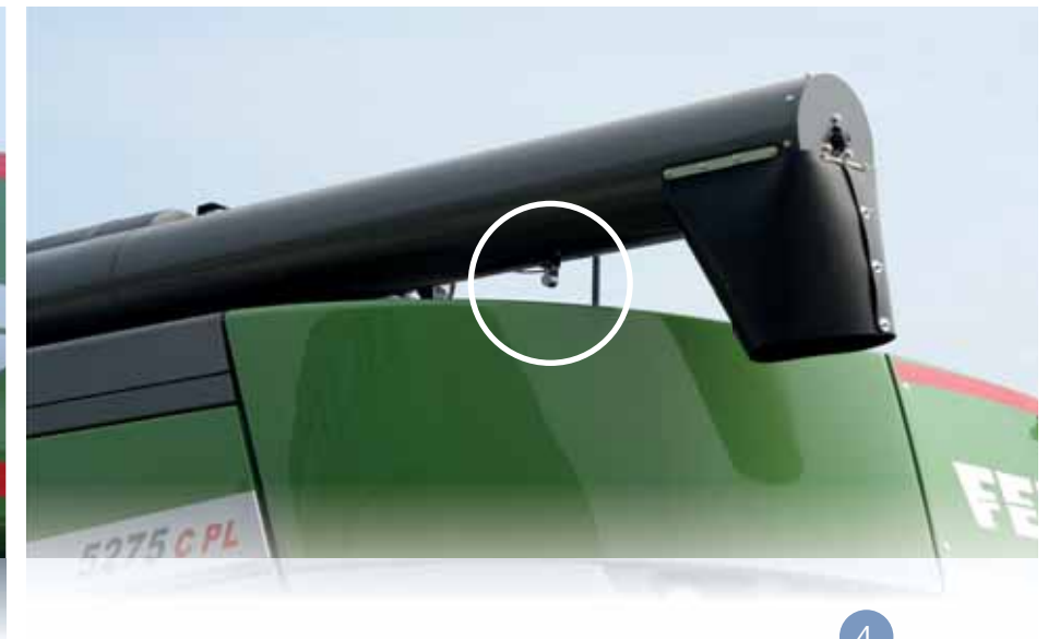
Top: Towing jaw monitoring during coupling Left: Rear view camera Right: Camera on the spout
