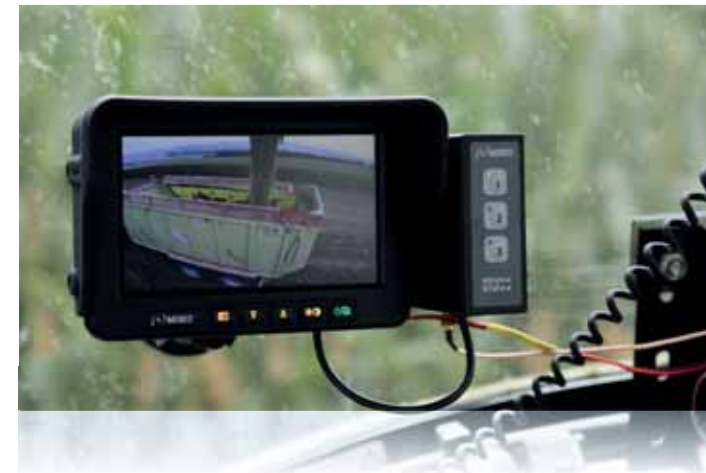
Bottom: Monitor with radio receiver in the support tractor's cab
