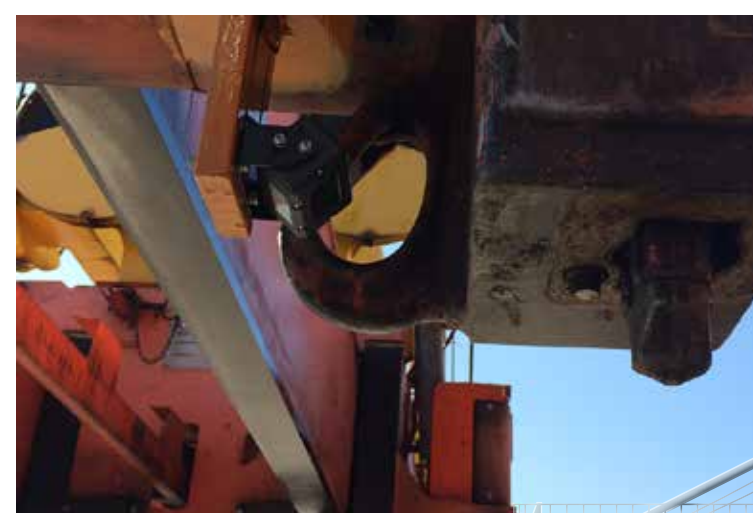
Twistlock camera in use during container handling.
