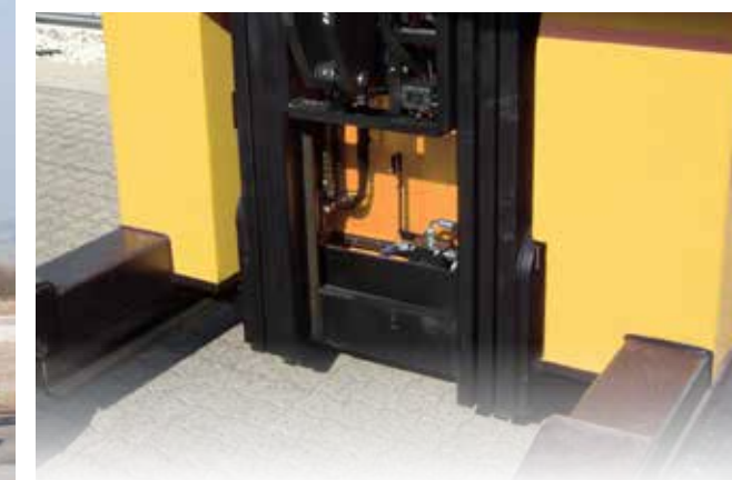
Motec mast or fork carrier camera – always level with the load.
