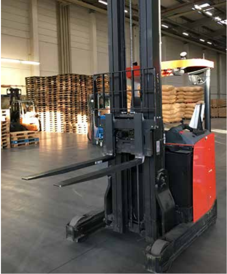
The fork camera on the reach truck allows the view onto both forks.
