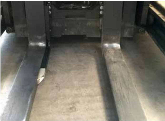
The fork camera on the reach truck allows the view onto both forks.
