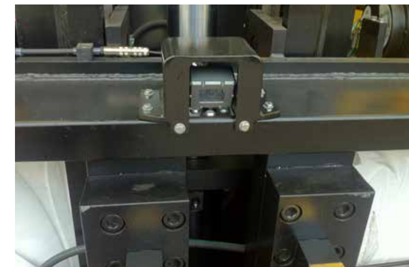
A carriage mounted camera is lifted simultaneously with the load.
