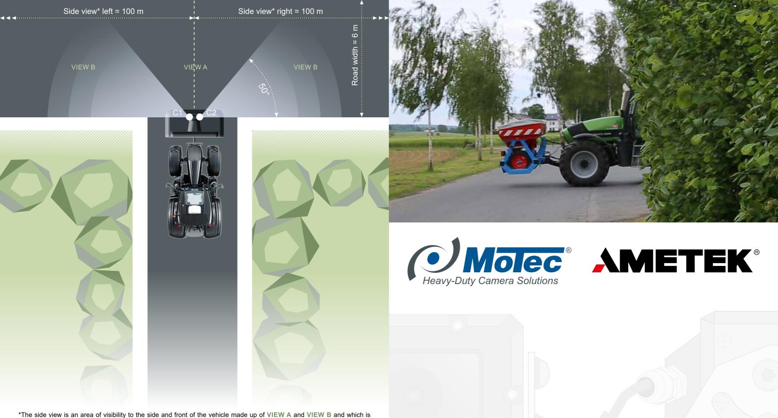
\*The side view is an area of visibility to the side and front of the vehicle made up of **VIEW A** and **VIEW B** and which is covered by the use of indirect visibility equipment (e. g. VKMS) combined with the direct vision of the vehicle driver.
